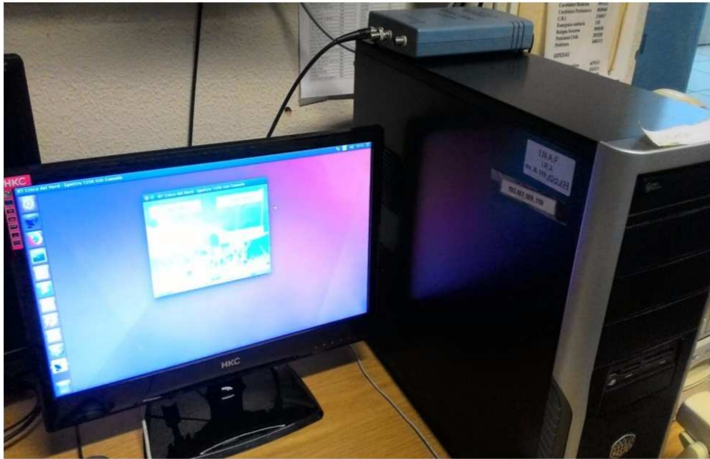
Fig. 1. Photo of the first pilot project spectrometer composed by a PC that host on the top of case the USB Oscilloscope.
