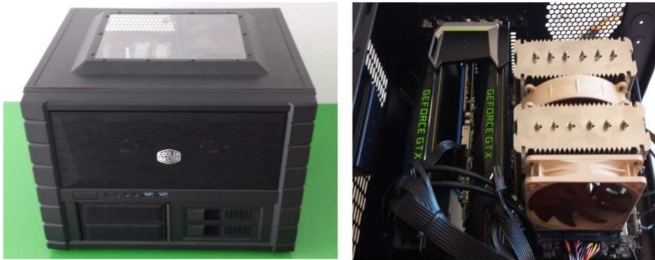
Fig. 6. Photos of the externals (on the left) and the internals (on the right) of the new spectrometer's prototype. In the right photo from the left, the second GPU, the DAQ board, the first GPU and the CPU's cooler system.
