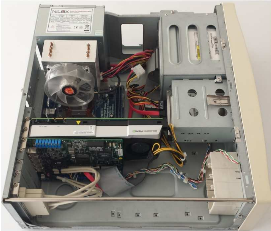
Fig. 2. Photo of the internals of second pilot project spectrometer. From the bottom the first add on board is the DAQ and the second is the NVIDIA Quadro 5000 GPU.
